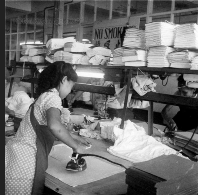
Cotton textile industry. Completed singlets are ironed and backed up with cardboard and packed in cartons. 1956.
